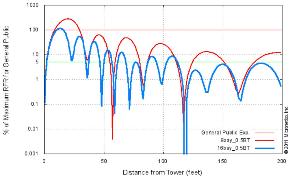
This plot shows the same 16 bay antenna (**Blue plot**) compared to a 8 bay antenna (**Red plot**) – 75 feet above the ground at 200 kW. The last grazing lobe of the 8 bay antenna leaves even a larger RFR hotspot near the tower.
