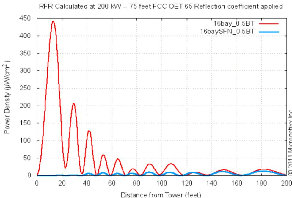
The graph below shows the MPE of the same two 16 bay antennas at 200 kW and 75 feet up. The red trace is a standard slot antenna, the blue trace is the Micronetixx low RFR antenna.
