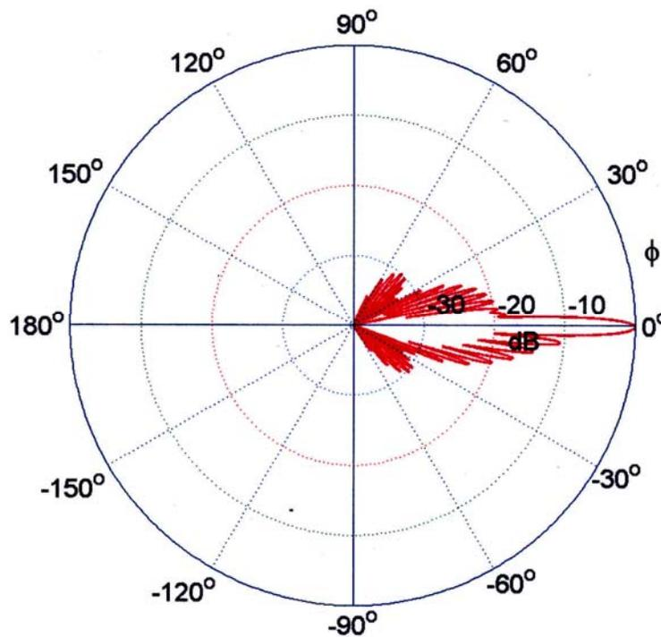
A polar plot of a 18 bay Micronetixx low RFR slot antenna, with 1 degree of beam tilt and 10% first null fill.
