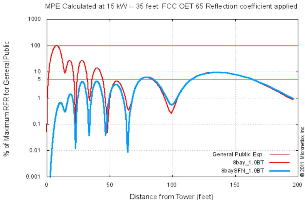
The plot below is a comparison of a 16 bay standard slot antenna (Red plot) and a 16 bay Micronetixx low RFR antenna (Blue plot).
