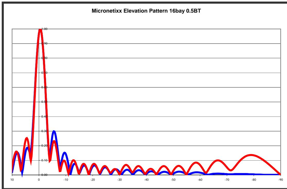
The graph below show the power density of the two antennas with an ERP of 200 kW and 75 feet up. The red plot is the standard slot antenna, the blue plot is the Micronetixx low RFR antenna.
