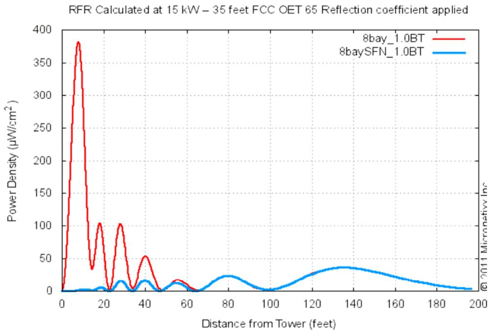
The graph above is the power density of the two 8 bay antennas mounted 35 feet up with an ERP of 15 kW. The red plot is the standard antenna, the blue plot a Micronetixx low RFR antenna.
