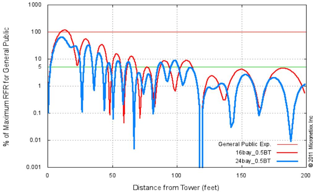
The plot above shows the MPE of the 200 kW station with a center of radiation 75 feet above ground. The **red plot** is the 16 bay antenna, the **blue plot** is the 24 bay antenna. The major grazing lobes about  $-80$  degrees down is on the left of the plot.
