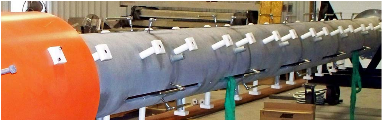
6 Bay TPV Top Mount Circular Polarized Top Mount Antenna With Radome Removed
